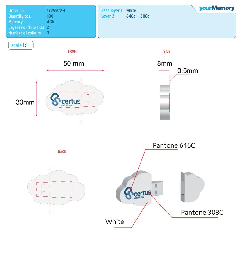
On the same layer, differents colours must be separated by a separation gap.
